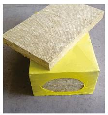
**SUNR**©CK® Resin Bonded (RB) Rigid Stonewool Slabs are designed for thermal and acoustical insulation of flat or slightly curved surfaces. They are efficiently used in Under Deck Insulation, Air Conditioning Duct Insulation, Sound Proofing of Auditoriums, Conference halls, Stadiums, Airports, Furnaces, Ovens, Cable Ducts, Tanks, Autoclaves and Chimneys, DG sets, Solar panels etc.
